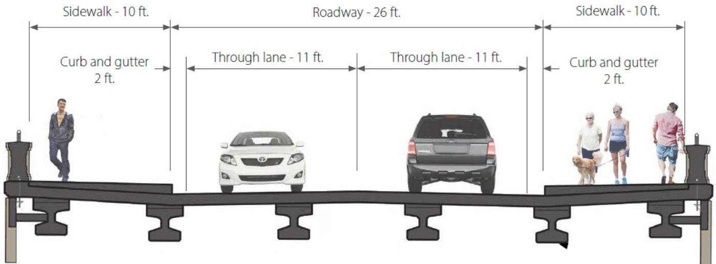
*The new bridge will feature 11-foot travel lanes in each direction for people driving and 10-foot sidewalks on both sides of the bridges to provide a wider space for people walking and rolling.*
