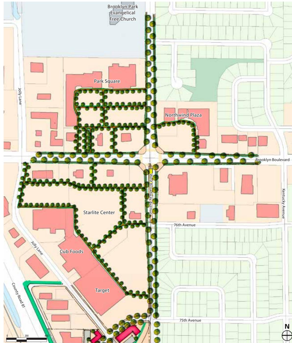
Fig. 38 PEDESTRIAN CONNECTIONS FOR BROOKLYN BOULEVARD STATION AREA
