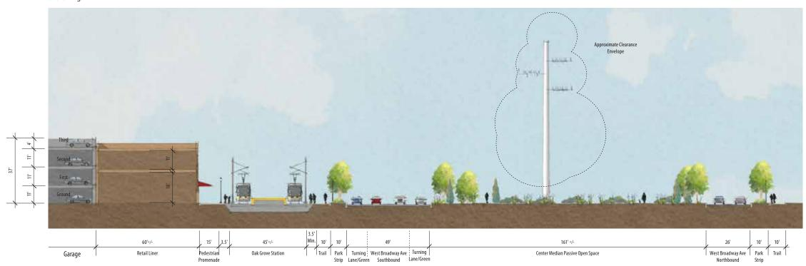
Fig. 53 WEST BROADWAY AVENUE SECTION AT LRT STATION The Grand Boulevard sets the primary address for development and transit.
