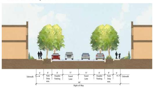
Fig. 51 TWO-WAY STREET WITH PARKING ON BOTH SIDES Moderate-scale street providing secondary access within large parcels where on-street parking is required. It accommodates on-street parking on both sides.
