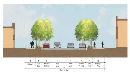
Fig. 48 TWO-WAY STREET WITH MULTI-PURPOSE PATH ON ONE SIDE This street is designed as a 30 mile per hour primary section for the Oak Grove loop road. On-street parking is permitted on both sides. A Class 1 bike lane on one side will act as a collector for the regional trail network.
