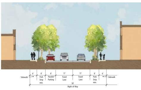
Fig. 52 TWO-WAY STREET WITH ONE SIDE PARKING Pedestrian-friendly small-scale street for local access where on-street parking demand is minimal. This street section may also be used to subdivide large development parcels.
