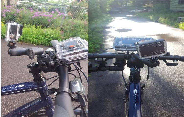
*Figure 1. C3FT Bike Mounted Radar and GoPro*
