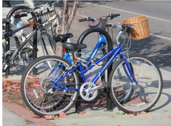
Figure 40 Wave Rack (Not Recommended)
