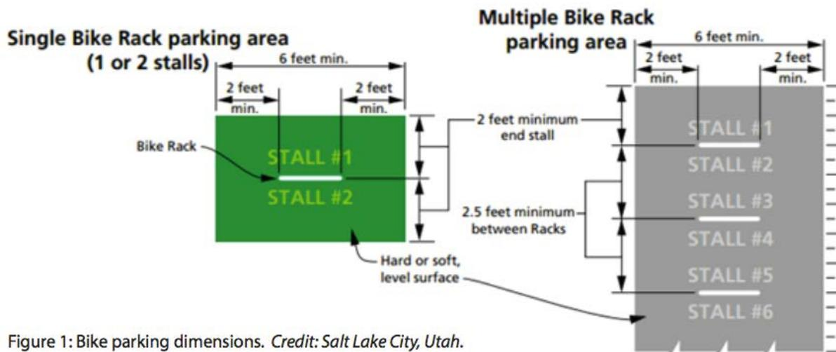
Figure 1: Bike parking dimensions. Credit: Salt Lake City, Utah.
