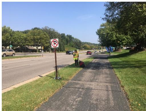
In locations with a shoulder or bicycle lane, tubes are placed across the shoulder or bike lane. In the absence of a dedicated bicycle facility, tubes are placed across the entire rightmost traffic lane. In locations with an existing off-street trail adjacent to the roadway, tubes are placed across the trail.
