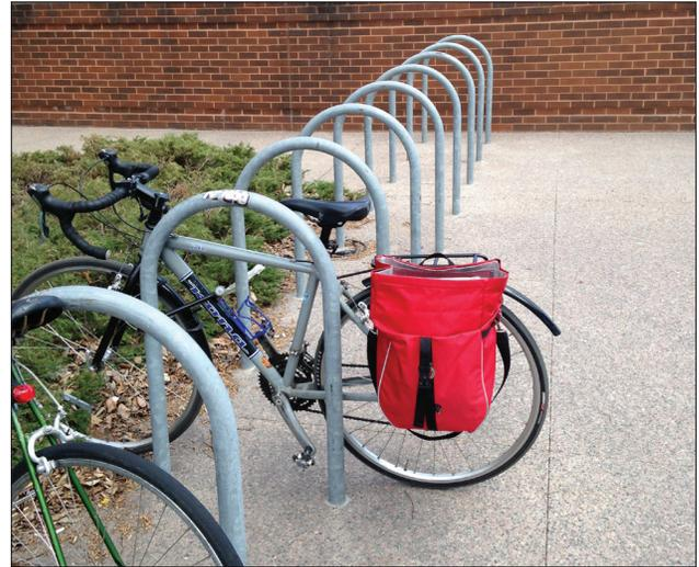
**Recommended — Inverted U or arc:** Can stand alone for curbside use or multiple racks can be installed for high density uses in bike corrals.
