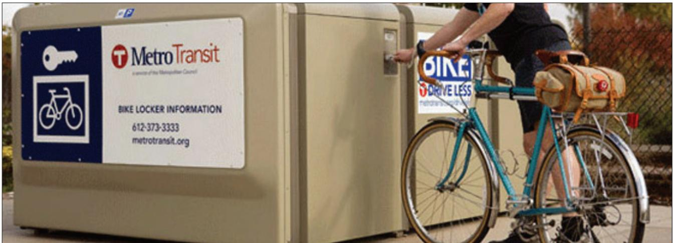
**Discouraged in many situations— Bike lockers:** Inefficient in terms of both cost and space. Bike lockers may be appropriate in low density areas if fewer than six long-term bicycle parking spots are needed. If lockers are used, electronic lockers (first-come, first-served with key card access) are strongly preferred over lockers leased to individuals. Bike lockers should be within 100 feet of the main building entrance or destination.
