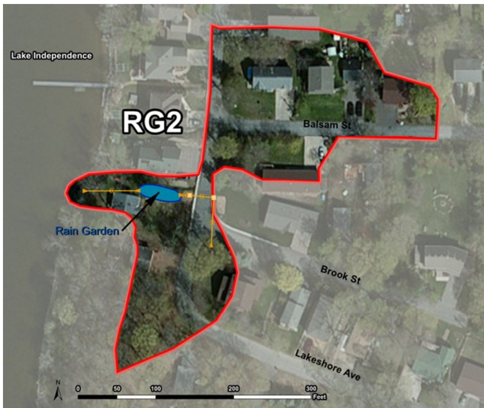
Figure 7U: Drainage area and location map
