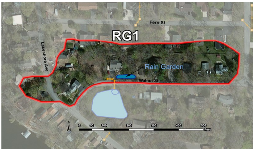
Figure 5U: Drainage area and locational map. Orange lines indicate existing drainage pipes
