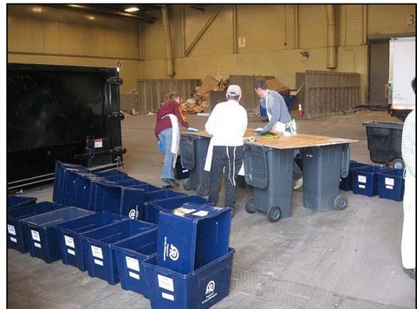
After waste is sorted, each container is weighed and that data is recorded. The final step in the design is an area designated for waste that has been sorted, weighed and is now ready for disposal.
