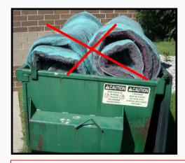
Nonhazardous paint booth filters are improperly stored outside in an uncovered dumpster. These filters can contaminate stormwater, so they represent a significant material. Read below.
