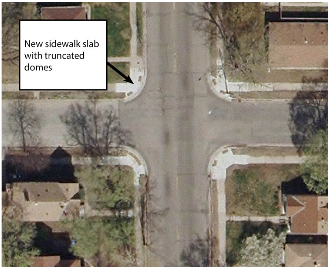
FIGURE 6-2: TYPICAL INTERSECTION UPGRADE
