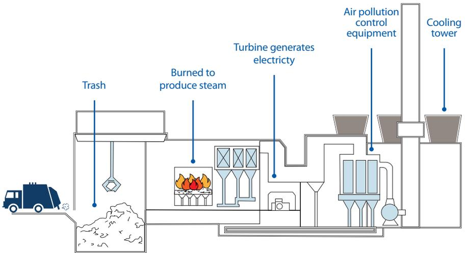
A portion of the steam provides heating and cooling to the downtown Minneapolis district energy system and Target Field. In fact, heat from HERC works to green up the ballpark turf before the Twins home opener in April and melt the snow at Target Field Station plaza all winter long.
