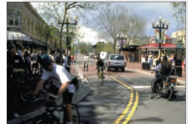
This narrowed street in Boulder, Colorado, successfully accommodates bicycles and a pedestrian crossing, while calming traffic.
