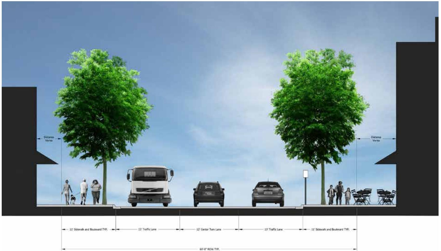
Figure 14: Recommended roadway section west of Central Avenue NE
