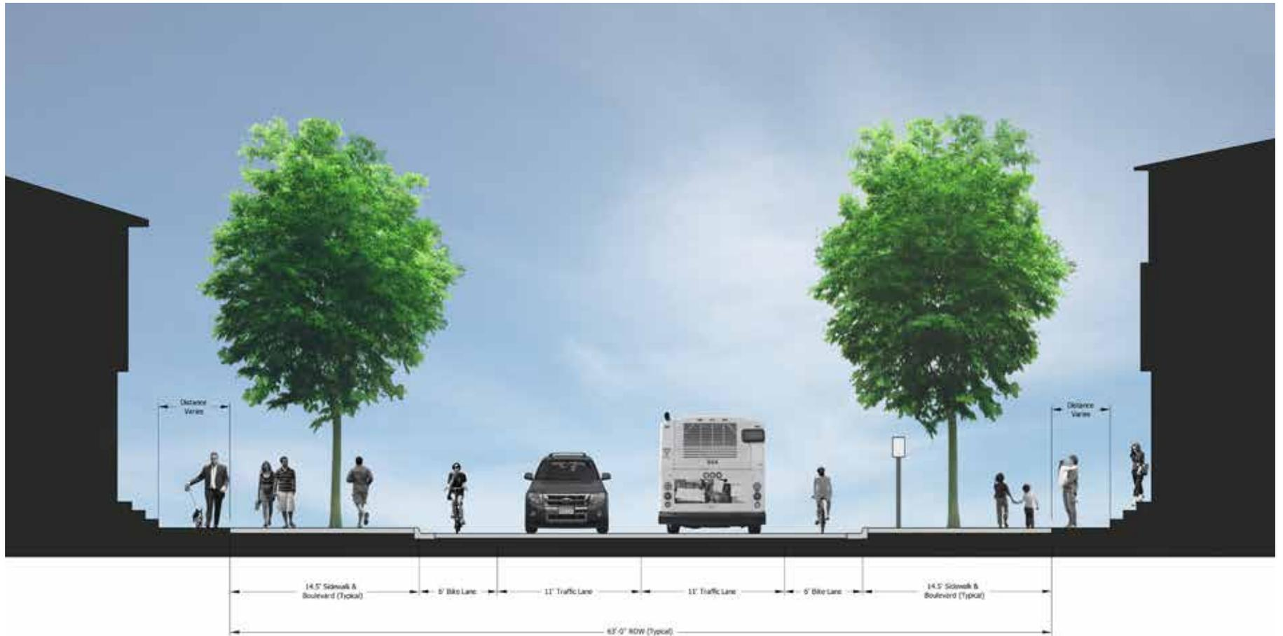
Figure 15: Recommended roadway section east of Central Avenue NE
