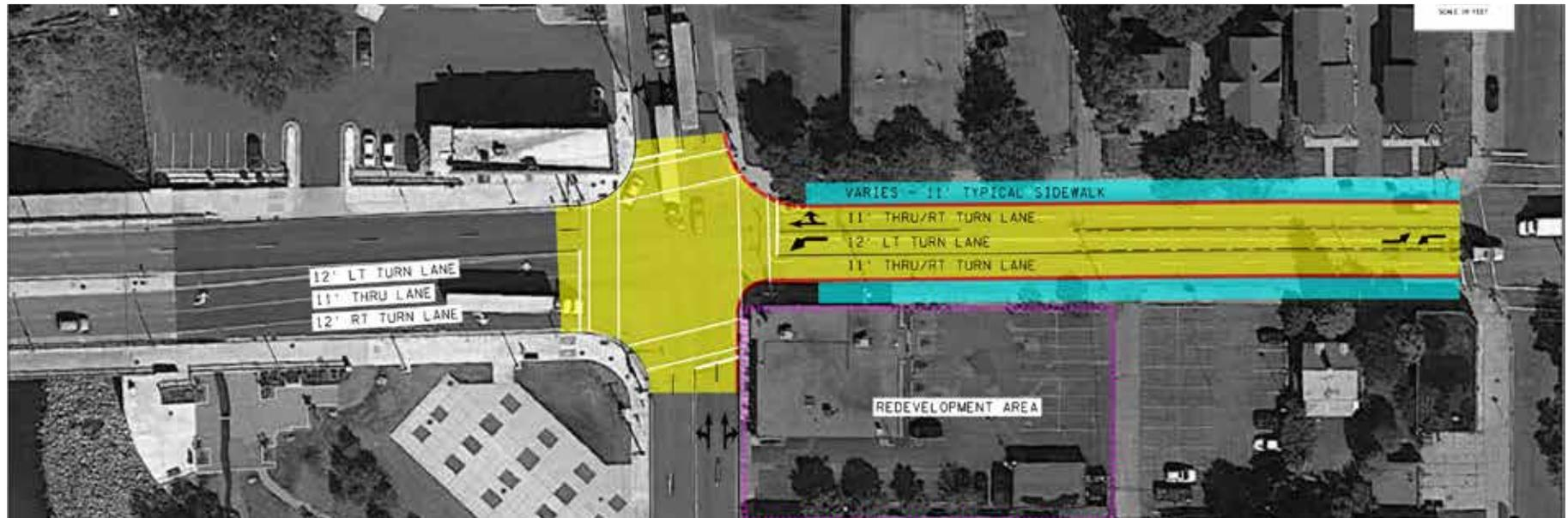
Figure 16: Recommended Improvements – Lowry Avenue NE at Marshall Street NE
